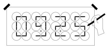
Drill the holes in the wall dimensioned to fit the wall anchors properly. Then, place the wall anchors and fix the hanging plate with the provided screws and washers.
