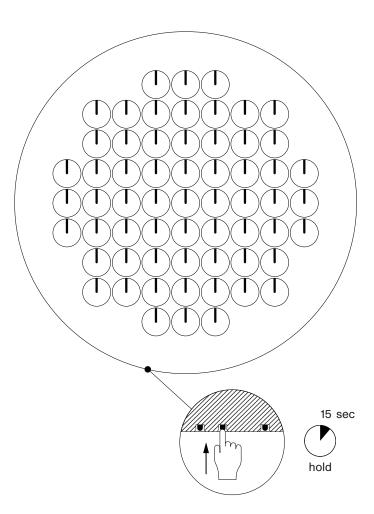
5.6 Power off the Artwork To power off the A million Times artwork first stop the artwork by pressing any of the buttons for a minimum of 15 seconds. Once all the hands are pointing up to 12:00, turn off the power switch located on the MC module at the back of the artwork. See section 5.1.2 for directions on accessing the MC module without removing the artwork from the wall.
